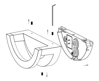
Remove the screws and open the back plate.
