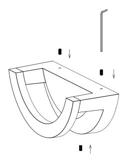
Lock the screws to fix the lamp.
