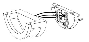
Fix the connector in correct position on back plate.
