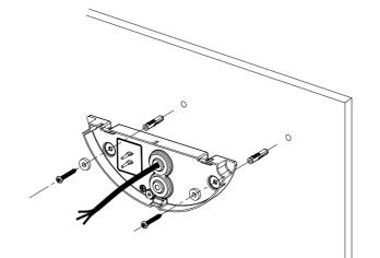
Wire through the waterproof rubber mat, fix the back plate on surface.
